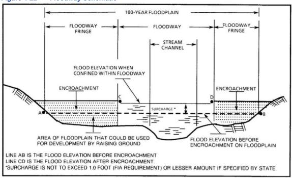
Figure 4-22 Floodway Schematic
